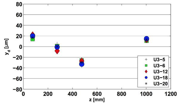
Figure 3: Relative displacements of the upstream magnets within five example U3 magnet blocks with respect to a linear fit of the displacements as a function of longitudinal position.
