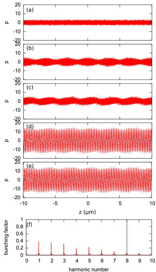
Figure 4: Numerical simulations of the longitudinal phase-space: (a) initial condition, (b) after laser heater, (c) assuming dispersion along the linac, (d) after seed modulation and (e) after the dispersive section. (f) corresponds to the bunching factor at the end, i.e. of the phase-space in (e).
