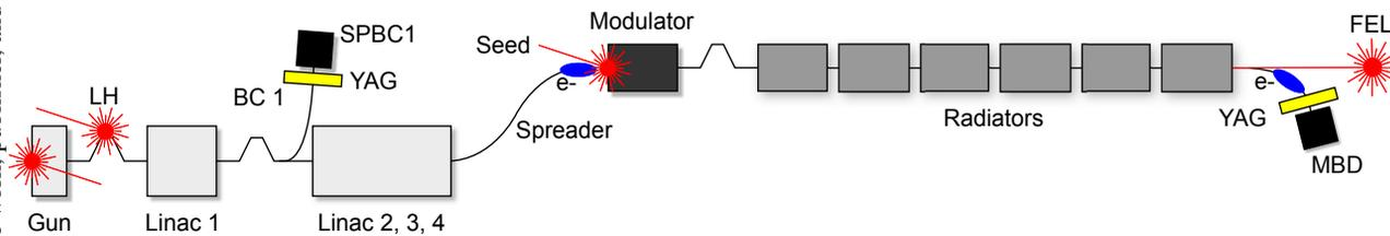
Figure 1: FERMI FEL-1 layout: Electron bunches are extracted from the photoinjector (Gun), propagate through the laser heater section (LH) and are then compressed in the bunch compressor (BC1). After being accelerated up to 1.5 GeV, they are sent to the FEL-1 undulators.
