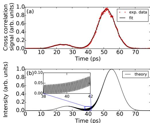
Figure 2: Laser heater pulse: (a) measured cross-correlation signal and (b) theoretical LH pulse shape. The beating region is localised in between the two pulses (inset).
