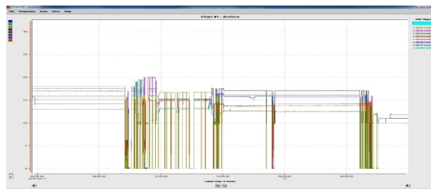
Figure 5: Gradient stability of cavities in C100-0 over 30 hours. Cavities are much quieter between 5PM and 7AM.
