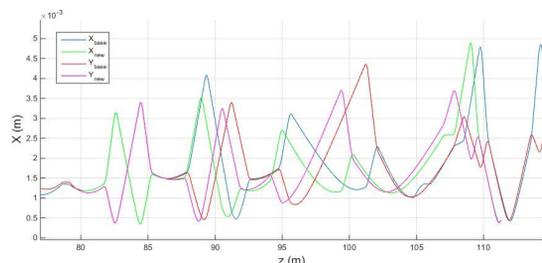
Figure 7: Transverse beam RMS size along LS1 in baseline and new rebuncher design (Criterion 2)
