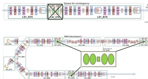
Figure 2: New lattice design with a single type of 4-cavity-QWR rebuncher (Criterion 1) [2].
