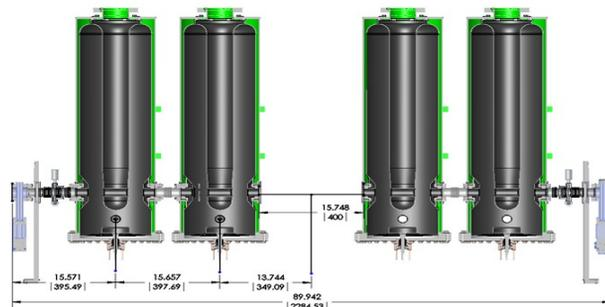
Figure 1: Mechanical drawing of the new 4-cavity-QWR rebuncher.
