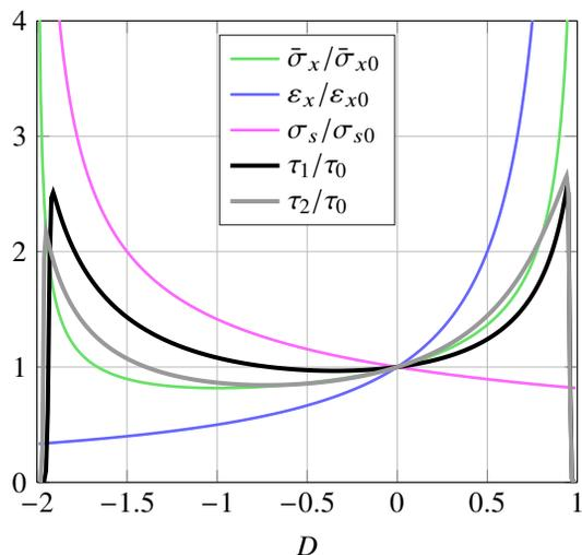
Figure 2: Average bunch width around the ring  $\bar{\sigma}_x$ , hor. emittance  $\epsilon_x$ , bunch length  $\sigma_s$  and lifetime  $\tau_{1/2}$  as a function of damping partition  $D$ , divided by corresponding  $D = 0$  values. Lifetime calculated for:  $\tau_1$ : constant vertical beam size  $\sigma_y(D) = \text{const.}$ ;  $\tau_2$ : for constant emittance coupling  $\sigma_y(D) \neq \text{const.}$ .
