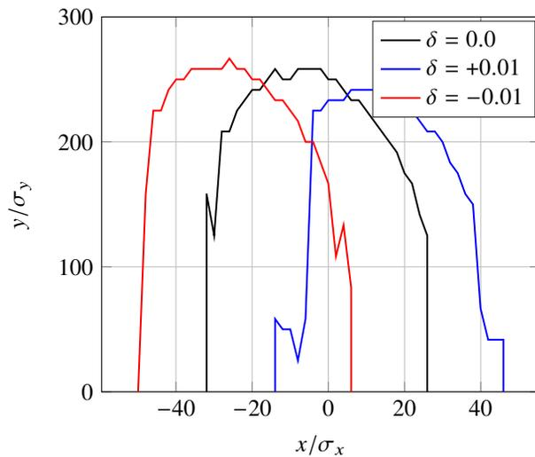
Figure 7: Dynamic aperture for the MLS with Robinson Wiggler calculated for different energy deviations.  $\sigma_x = 701 \mu\text{m}$ ,  $\sigma_y = 36 \mu\text{m}$ ,  $\eta_x = 0.54$  m
