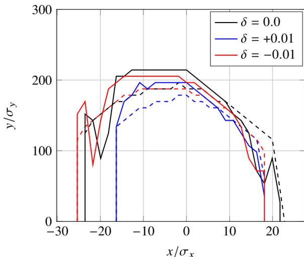
Figure 6: Dynamic aperture for the MLS without Robinson Wiggler calculated with MAD-X (dashed) and the self-written code (solid) for different energy deviations.  $\sigma_x = 966 \mu\text{m}$ ,  $\sigma_y = 42 \mu\text{m}$ ,  $\eta_x = 0.17$  m
