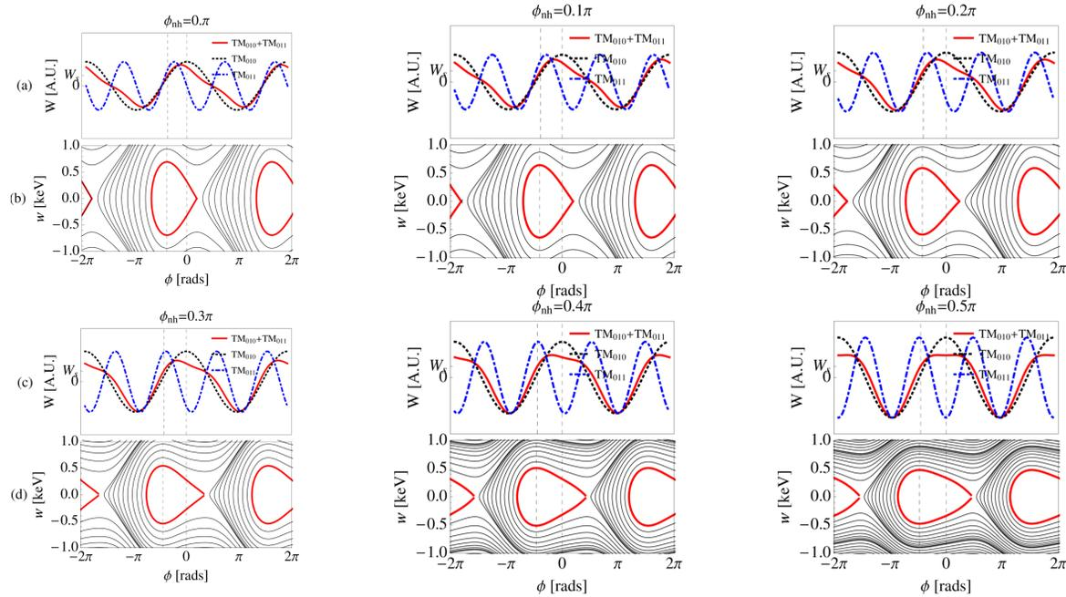
Figure 2: Phase space plots for a cavity exciting both the  $TM_{010}$  and  $TM_{011}$  modes. A phase shift is gradually applied to the  $TM_{011}$  mode and the gradient is kept constant for each step. For all steps,  $\alpha = 0.222$ . Rows (a) and (c) show the energy gain of a traversing particle as a function of its initial phase offset. Rows (b) and (d) show the phase space contours, with the separatrix marked in red.
