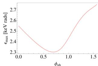
Figure 3: Acceptance of the accelerating bucket in a second harmonic cavity with  $\alpha = 0.222$  as a function of  $\phi_{nh}$ .
