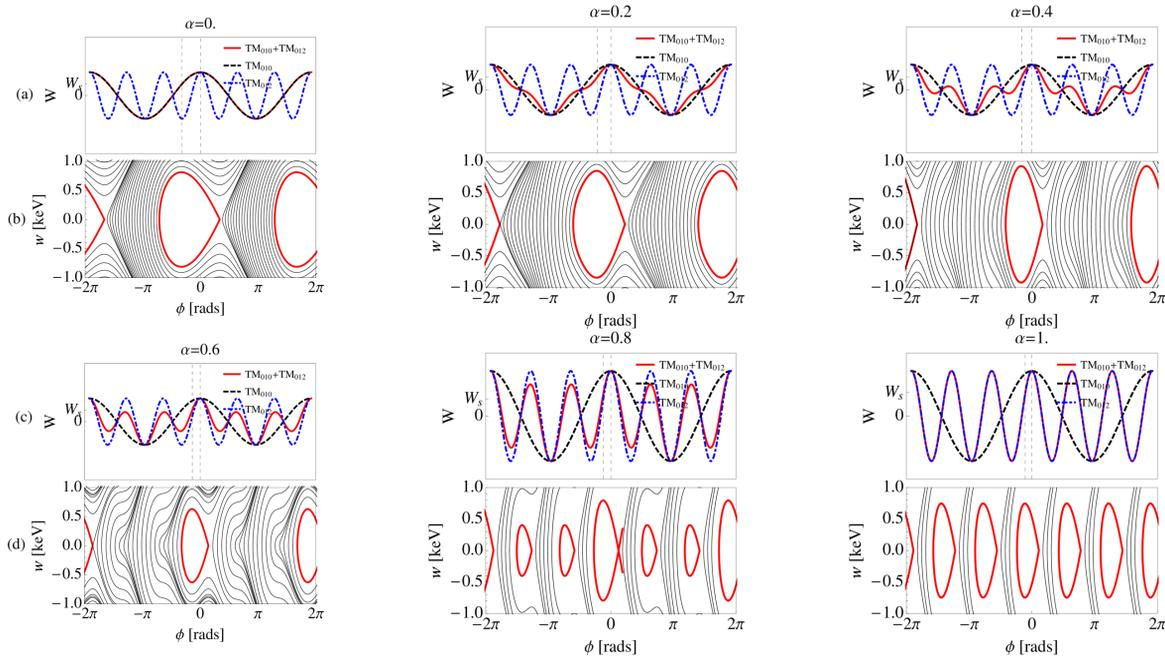
Figure 4: Phase space plots for a cavity exciting both the  $TM_{010}$  and  $TM_{012}$  modes.  $\alpha$  is varied to determine at what harmonic field strength secondary buckets begin to emerge. Rows (a) and (c) show the energy gain of a traversing particle as a function of its initial phase offset. Rows (b) and (d) show the phase space contours, with the separatrix marked in red.
