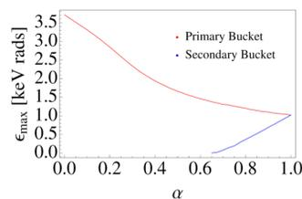
Figure 5: Acceptance of the accelerating bucket as a function of  $\alpha$ . The red line is the primary bucket and the blue line is for the secondary buckets.
