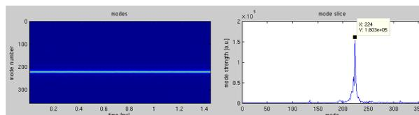
Figure 1: Instability Mode analysis of IVU05 at 6.4mm gap. Mode 224 is the strongest mode, but the neighbouring modes are also excited, indicating a resonance with width of multiple revolution harmonics.
