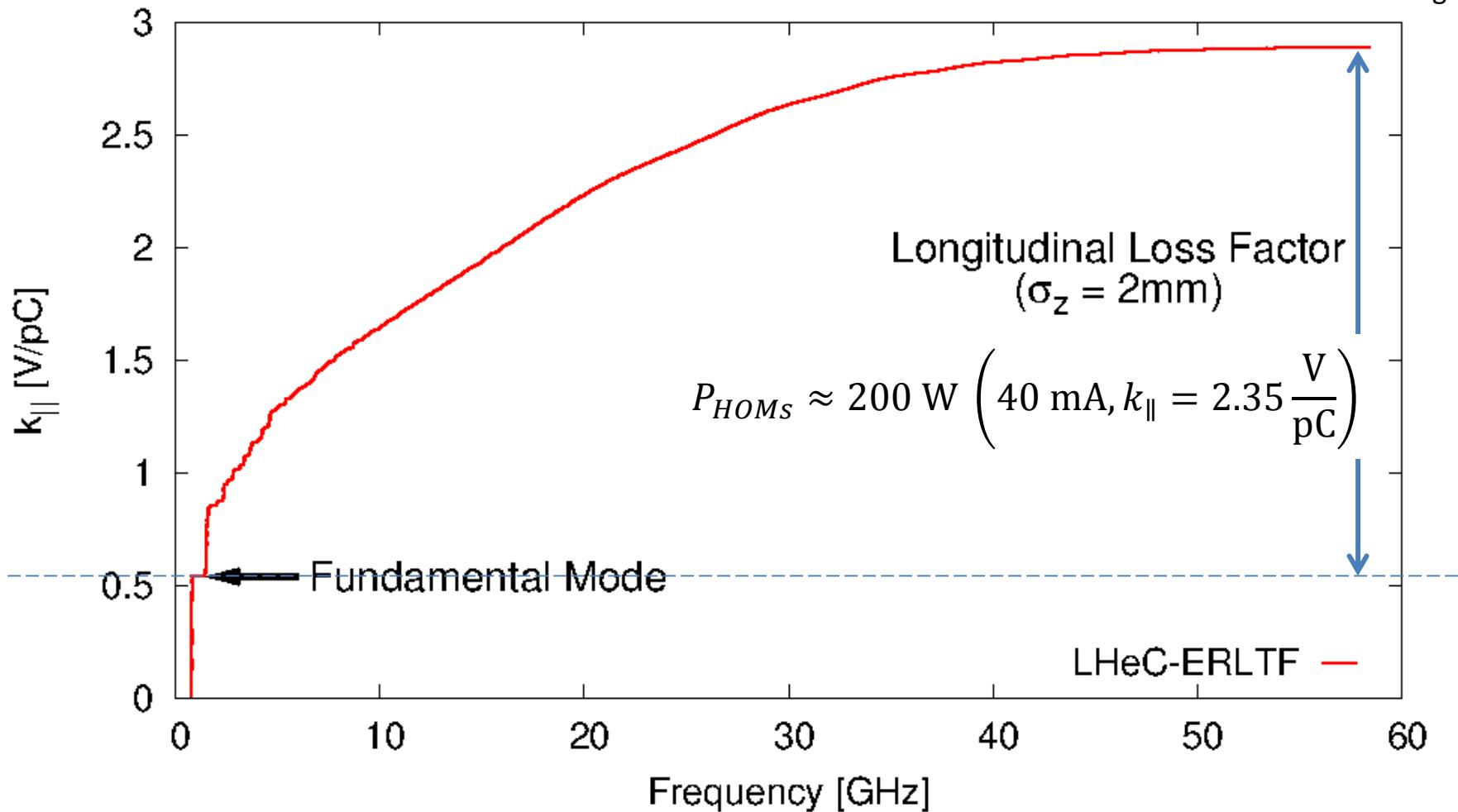
Note: with 13 mA injected, the total current for HOM excitation can be 80 mA!
