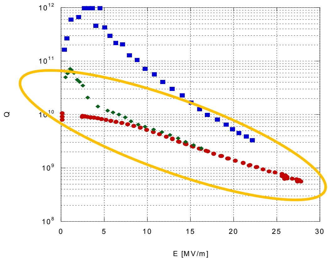
With HiPIMS at this early stage we are currently **at the level of the best performing magnetron sputtering coatings**, for an equivalent surface preparation (SUBU vs EP)
