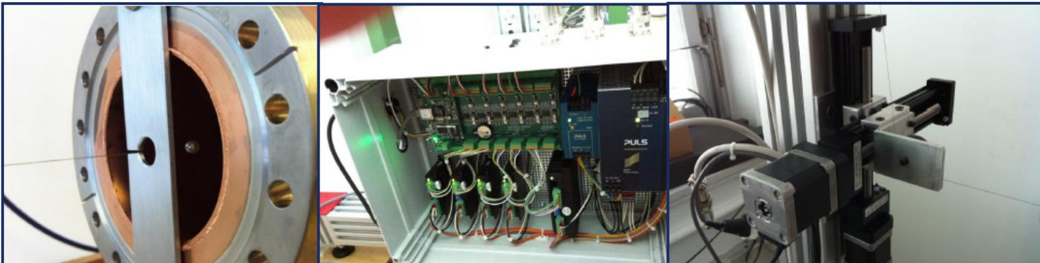
Bead-pull measurement setup for field mapping
