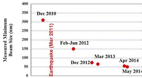
Figure 4: History of measured minimum beam size.
