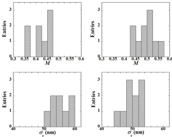
Figure 5: Two sets of consecutive beam size measurements. Top: Distributions of the IPBSM modulations with 174 degree mode. Bottom: Beam size distributions evaluated from the modulations, without systematic error correction (These represent upper limits of the beam sizes.). The bunch charges during the measurements were about 160 pC (left) and 90 pC (right). Data were taken on April 17 (left) and May 22 (right), 2014.
