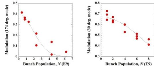
Figure 6: IPBSM modulation as function of bunch population. Measured with a crossing angle 174 degrees (left) and 30 degrees (right).
