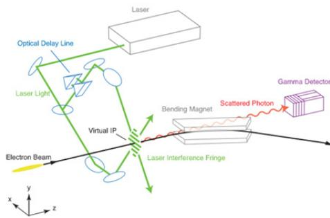
Figure 2: Beam size monitor at the focal point, called IPBSM, or Shintake Monitor [11].
