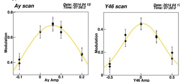
Figure 3: Examples online figures of knob scans. IPBSM modulations as functions of strengths of tuning knobs (a.u.). Left: A linear knob scan with IPBSM crossing angle 30 degrees. Right: A non-linear knob scan with IPBSM crossing angle 174 degrees. After each scan, “knob” was set at the peak of the fitted curve.
