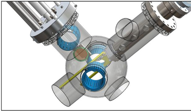
Figure 5: JLab FEL diagnostic module for LDR imaging and wire scanner transverse beam profile measurements with built-in impedance shield
