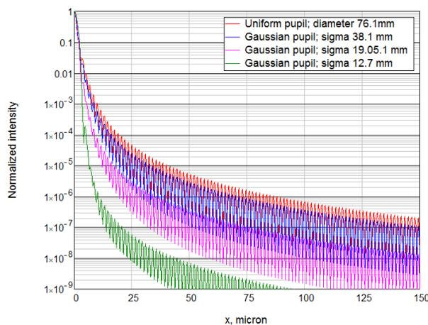
Figure 2: PSFs of uniform and Gaussian pupil functions.
