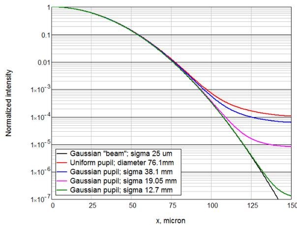
Figure 1: Gaussian distribution compared to its convolutions with PSFs from Figure 2.
