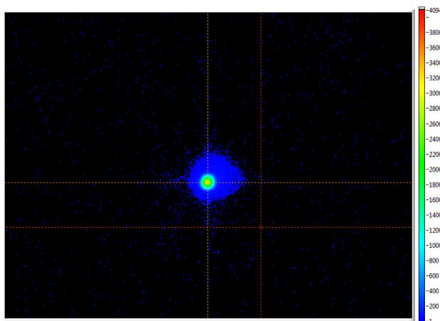
Figure 4: Pinhole image with Gaussian apodizer.
