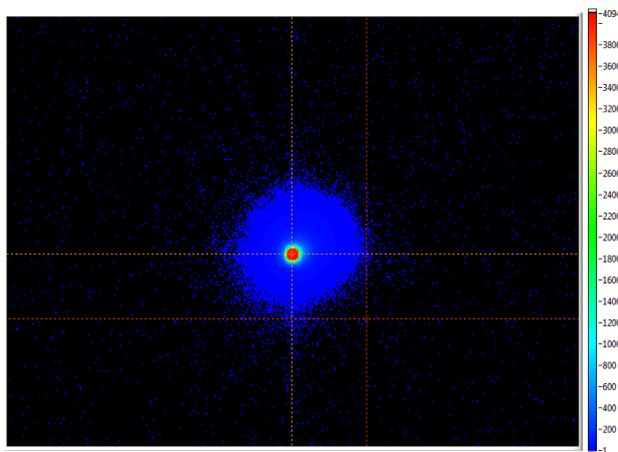
Figure 3: Pinhole image without an apodizer.
