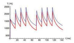
Figure 4: Peak foil temperatures evolution at the H<sup>-</sup> spot center derived from the 3D model (Eq. [2]) (continuous) and the 1D model (Eq. [5]) without heat conduction (dotted).
