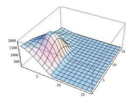
Figure 3: Peak temperature distribution at the Foil for the combined load from injected H<sup>-</sup> and circulating protons.
