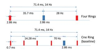
Figure 1: Pulse distribution for the 4-ring and the one-ring options: The upper part of the figure shows the 28 Hz pulsing of the linac with one proton (blue) and one  $H^-$  (red) pulse interleaved and the lower part shows the case where four 0.72 ms long pulses of  $H^-$  for neutrinos are followed by one 2.86 ms proton pulse for the neutrino spallation target.
