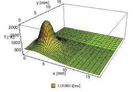
Figure 6: Foil temperatures evolution on the foil surface (x,y-directions). The time is that of the  $8^{th}$  injected spot 115 ms where the peak temperature of 2210 K is reached.
