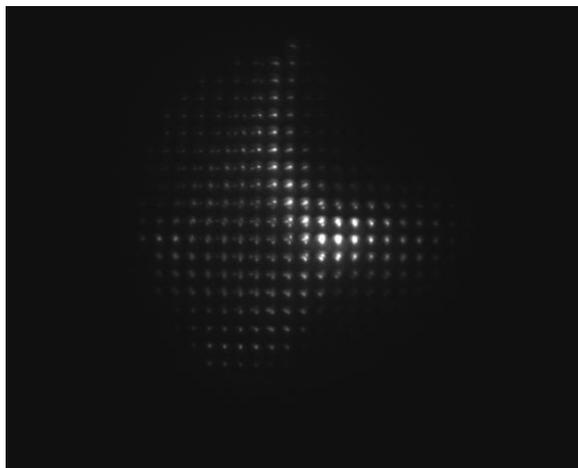
Figure 3: Pepper pot image captured from C<sup>4+</sup> ions at the pulse ion current of 12  $\mu\text{A}$  on the RFQ exit. The optical focus was set to the solenoid (Fig. 1), not to the pepper pot.
