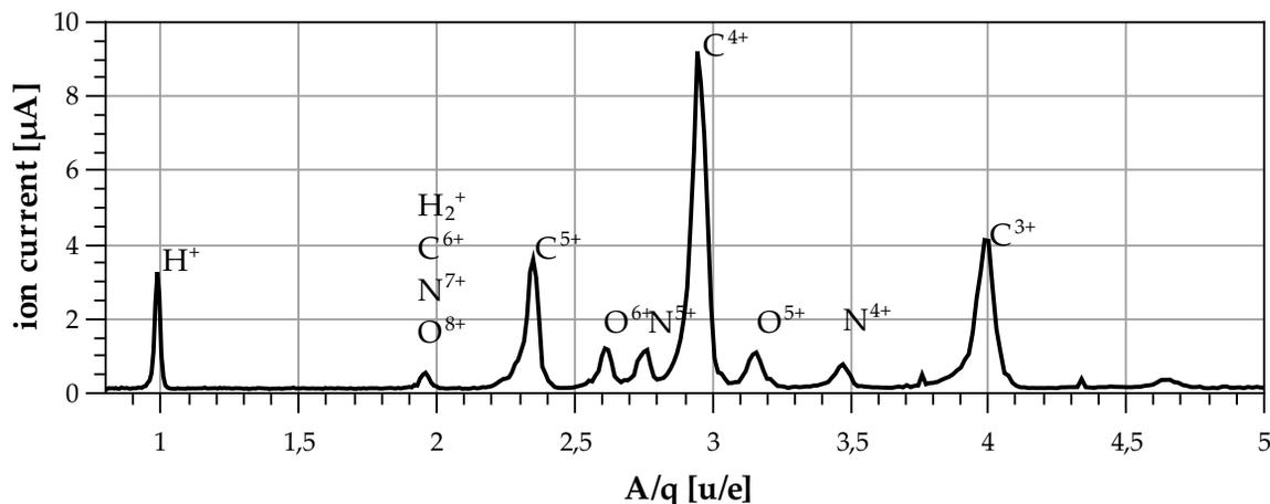
Figure 2: Ion spectrum with dominant C<sup>4+</sup> ion peak measured at Faraday cup 1 at a pressure of  $8 \times 10^{-8}$  mbar, an ionisation time  $t_{\text{ion}}$  of 15 ms, an electron beam current of 550 mA and an analyzing slit width of 10 mm. The fraction of C<sup>4+</sup> ions results in 26 %.
