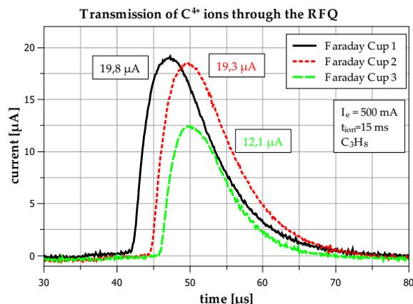
Figure 4: Transmission of a C<sup>4+</sup> ion pulse from Faraday cup 1 (black solid line) to Faraday cup 2 (red dotted line) passing the RFQ to Faraday cup 3 (green dashed line).
