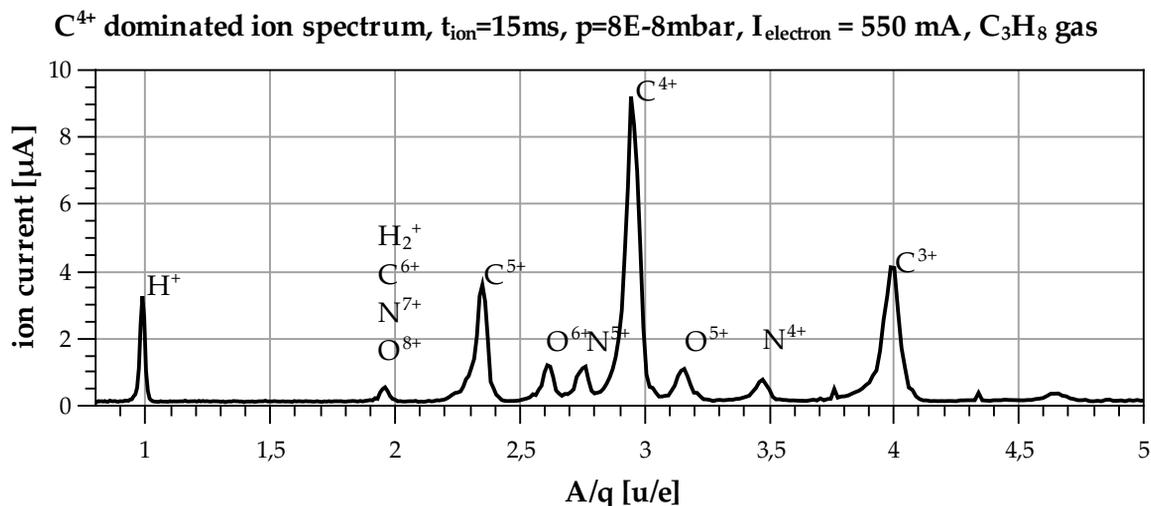
Figure 2: Ion spectrum with dominant C<sup>4+</sup> ion peak measured at Faraday cup 1 at a pressure of  $8 \times 10^{-8}$  mbar, an ionisation time  $t_{\text{ion}}$  of 15 ms, an electron beam current of 550 mA and an analyzing slit width of 10 mm. The fraction of C<sup>4+</sup> ions results in 26 %.
