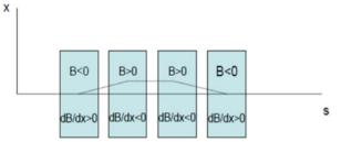
Figure1: There are four combined function magnet in one set of Robinson wiggler, the value of product of dipole and quadruple magnetic field in Robinson wiggler is negative ( $\frac{dB}{dx} < 0$ ), it's used to change damping partition number to achieve the goal of decreasing horizontal emittance.
