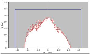
Figure 5: This figure shows the beam aperture with MRW by nonlinear optimization, the beam aperture size is about 20mm.
