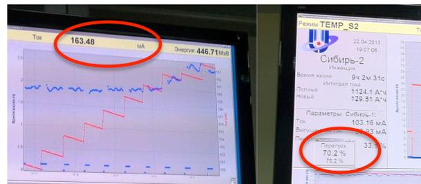
Figure 8: Current and injection efficiency with new generators.
