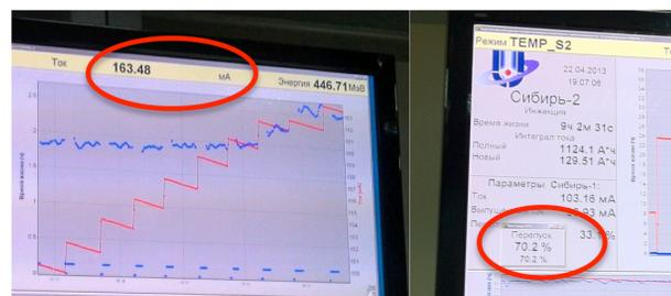
Figure 8: Current and injection efficiency with new generators.
