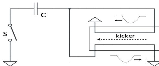
Figure 4: Simplified scheme of the new generator.
