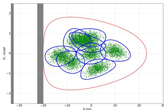
Figure 7: Phase trajectory of one stored bunch on the septum magnet azimuth during 7 turns.
