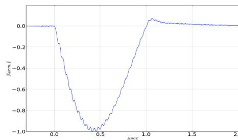
Figure 5: Digital oscillogram of the current pulse on the kicker.
