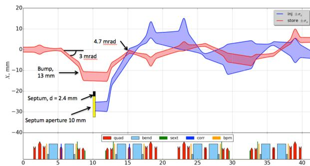
Figure 3: Trajectories of injected and stored beams in the moment injection, with sextupole influence.
