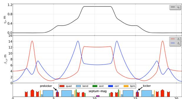
Figure 2: Siberia-2 optical functions.
