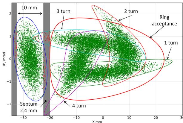
Figure 6: Phase trajectory of injected beams on the septum magnet azimuth. Ellipse and particles distribution are  $\pm 3(\sigma_x, \sigma_{x'})$ .
