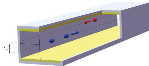
Figure 1: Conceptual design of a beam-driven short period FEL undulator.
