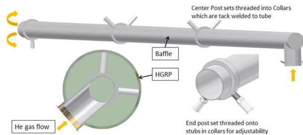
Figure 6: Baffle tube supported with spoke rods in HRGP, required for the prototype module, only.
