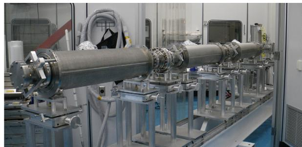
Figure 4: String assembly inside the cleanroom- 3 cavities being already connected.
