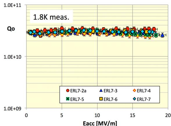
Figure 3: Vertical test results for all 6 ERL cavities. All cavities exceeded the design specifications for the ERL ( $Q=2 \cdot 10^{10}$  at 1.8 K). The reproducibility of the results, gained without any reprocessing of a cavity, is remarkable.
