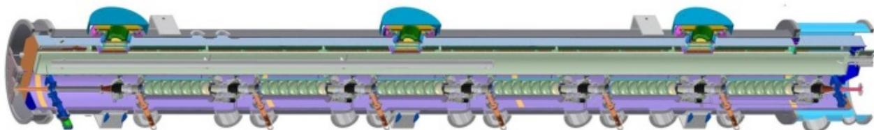
Figure 1: CAD model of the Cornell ERL Main Linac Cryomodule (MLC) prototype. It has 6 cavities (7-cells, 1.3 GHz, BBU-optimized shape) and beam line higher order mode absorbers.
