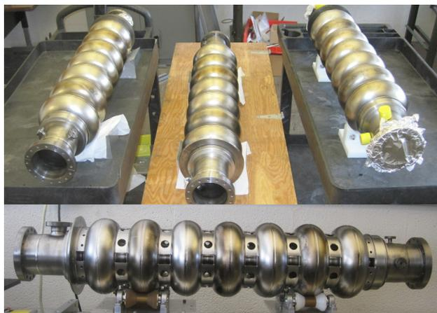
Figure 2: Picture of the superconducting cavities for the MLC. Six were built in-house, three of them have stiffening rings.
