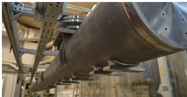
Figure 7: Assembly frame, supporting the HGRP which acts as a strongback for all beam line components, hung under the precision machined mounting feet.
