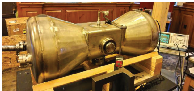
Figure 7: Helium vessel leak check setup.
