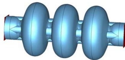
Figure 3: Example for design studies based on TESLA cells to increase the cell-to-cell coupling and HOM propagation by fluted iris.
