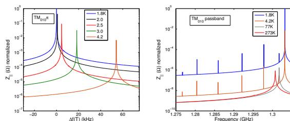
Figure 5: Impedance of the  $TM_{010}-\pi$  mode (left) and the  $TM_{010}$  passband for different temperature level accounting for frequency shifts by helium pressure and thermal shrinkage/expansion for the bERLinPro design.
