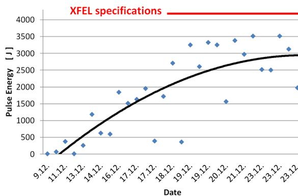
Figure 4: Gun conditioning energy over time.
