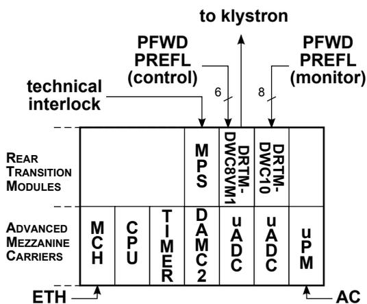
Figure 2: Schematic layout of the LLRF MTCA modules.
