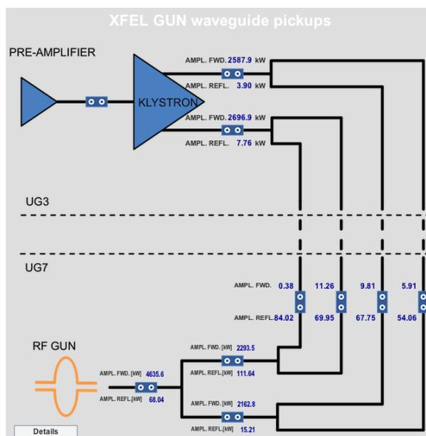
Figure 1: Gun RF distribution scheme and measurement points.
