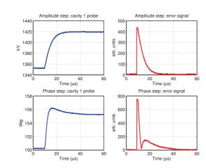
Figure 2: Closed-loop step response measurement.
