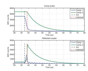
CC BY 3.0 licence (© 2014). Any distribution of this Figure 3: Example of a captured interlock event at ELSA, with an arc in cavity 1 triggering reflection interlock.
