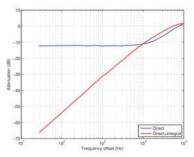
Figure 4: Internal network analyzer measurement showing error suppression with and without integrator.
