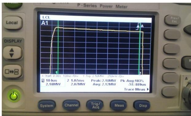
Figure 3: RF power meter showing 2MW RF output.
