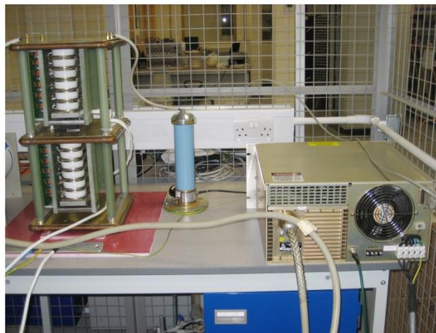
Figure 4: solid state crowbar under test at 38kV.
