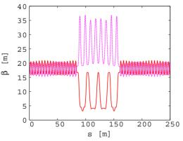
Figure 1: Horizonatl (red line) and vertical (pink one) betatron fuctions in the half of nuSTORM RFFAG ring.
