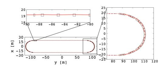
must 1 Figure 4:Layout of the ring with magnified cells in the production straight and in the arc together with muon closed orbits. The racetrack shape of the ring is dictated by the need of a high neutrino production efficiency.
