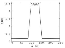
Figure 2: Dispersion fuctions in the half of nuSTORM RFFAG ring.
