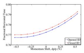
Figure 1: Results of multiple automated chromaticity scans enabled by the fully integrated tune readout. The blue curve represents the mean data of the scan with all insertion devices opened, whereas the red curve is the result with one insertion device closed. The statistical errors on the measured values are smaller than the size of the markers for each data point, demonstrating that changes to the machine state create tune shifts clearly resolved by the tune measurement method.
