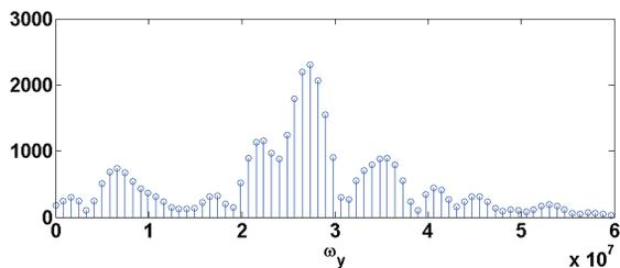
Figure 5: Oscillation frequency spectrum of the  $H_2$  ions in a drift. The ion charge density neutralizes the beam charge density.
