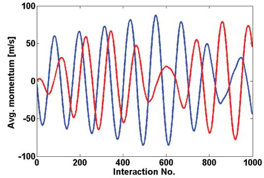
Figure 2: Average vertical (blue) and horizontal (red) velocity of the  $H_2$  ions during interaction with 1000 bunches in a quadrupole. The ion charge density is a quarter of the beam neutralization charge density.
