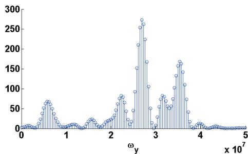
Figure 4: Oscillation frequency spectrum of  $H_2$  ions in a quadrupole. The ion charge density neutralizes the beam charge density.
