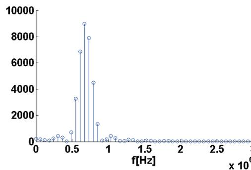
Figure 8: Oscillation frequency of iron ions interacting with 100 mA beam.
