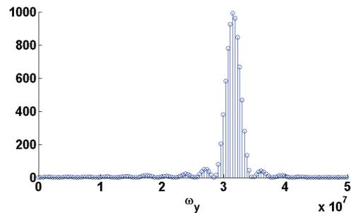
Figure 3: Oscillation frequency spectrum of the  $H_2$  ions in a quadrupole. The ion charge density is a quarter of the beam neutralization charge density.
