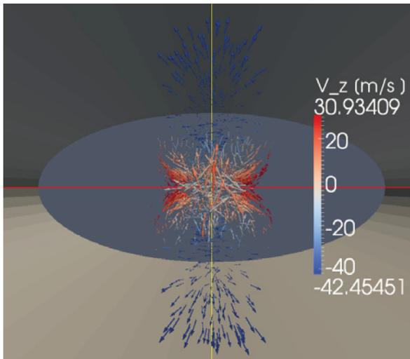
Figure 1: Ions oscillating in the quadrupole field receive a longitudinal component of the velocity.
