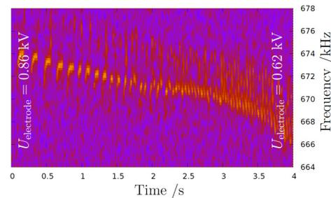
Figure 6: Influence of the clearing electrodes on the dynamic behaviour of the coherent tune of the horizontal instabilities. Measured at 1.2 GeV and 76 mA.
