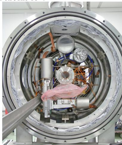
Figure 6: Front view of the SRF Gun II cryostat with both steppers—holding the SC solenoid—installed and fully equipped with their thermal anchors and magnetic shielding. (The magnetic shielding of the solenoid itself is not yet installed in this picture.)
