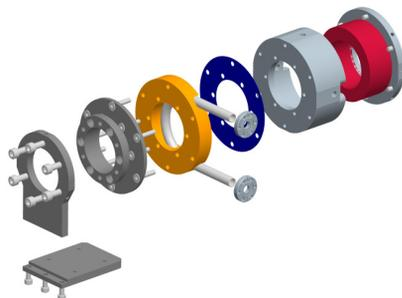
Figure 3: Exploded view of the superconducting solenoid, from left to right: Front plate with base plate, connector, copper cooler with helium pipe, indium disc, solenoid yoke, coil, yoke back plate.
