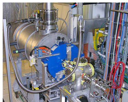
Figure 1: Picture of the Rossendorf SRF Gun I beam line including the cryostat in the back and the normal conducting solenoid (blue) at the injectors exit. The beam direction is to the lower right.
