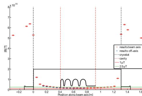
Figure 4: Combined results of measurements of the absolute magnetic field inside the cryostat. The red ticks represent two measurements done at different orientations of the cryostat, both measured along the beam axis. The blue marks show a measurement of the field on an axis through an off-axis hole in the shield, this is roughly at the position of the resonator's equator.
