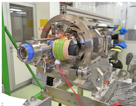
Figure 5: A coil made of copper wire, wrapped around one of the critical hand valves at the rear of the cavity string. The coil is operated by two power supplies, generating an altering, decreasing current.
