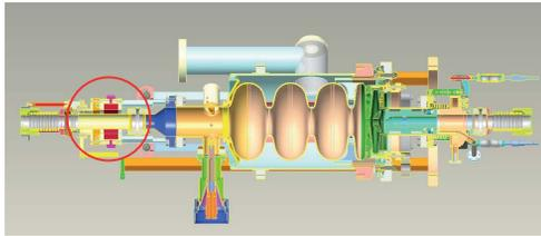
Figure 2: Drawing of the cavity string of the 3-1/2-cell resonator with highlighted position of the superconducting solenoid which is located about 70 cm from the cathode in the first half-cell.
