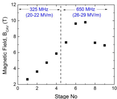
Figure 3: Axial magnetic field at the cavity edge for each cooling stage.
