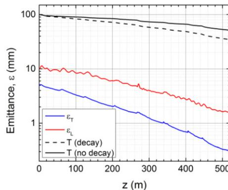
Figure 5: Cooling performance of a hybrid channel that uses LiH absorbers and gas filled cavities.
