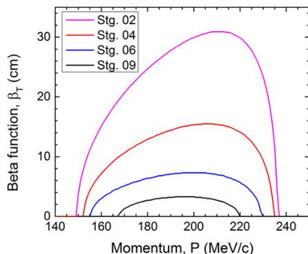
Figure 2: Momentum acceptance for different stages along the channel.
