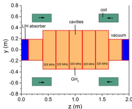
Figure 4: Schematic illustration of a hybrid channel cell with gas filled cavities for stage 2.
