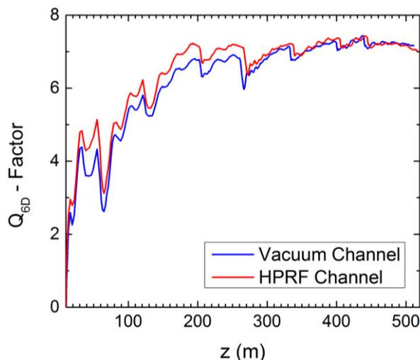
Figure 6: Quality factor, Q versus z for a channel with vacuum and gas-filled rf cavities. Both channels achieve same cooling efficiency along the channel.
