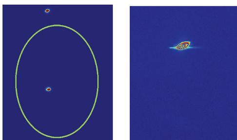
Figure 2: Left: bunch for FLASH1 (bottom) and bunch for FLASH2 (top) right before extraction septum. Right: bunch at FLASH2 dump screen. Beam dimensions are not to scale.
