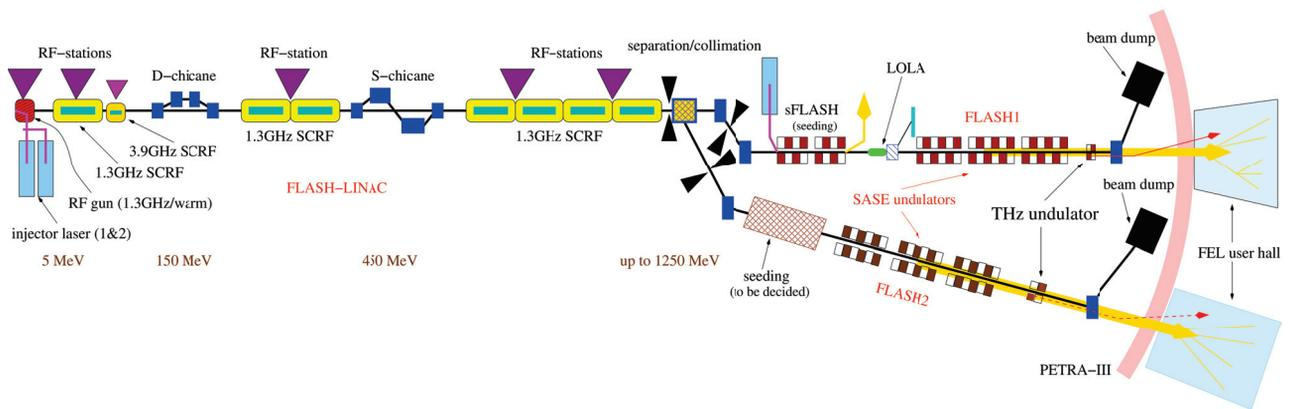
Figure 1: Schematic FLASH layout including beam lines FLASH1 and FLASH2.
