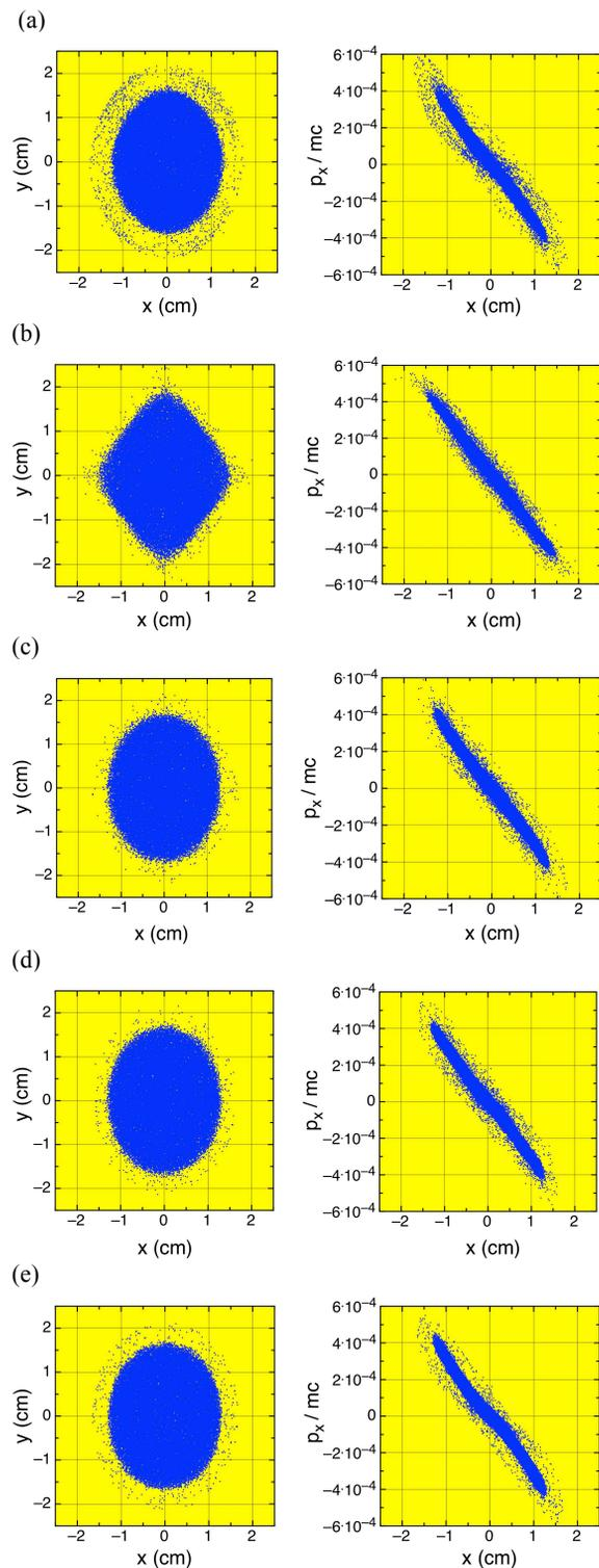
Figure 5: Particle distributions after 100 focusing periods: (a) pure quadrupole channel, (b) quadrupole-duodecapole channel with constant  $\eta = 0.0156$ , (c) quadrupole-duodecapole channel with initial  $\eta = 0.0177$  and  $N_{adiabatic} = 100$ , (d) quadrupole-duodecapole channel with initial  $\eta = 0.0182$  and  $N_{adiabatic} = 50$ , (e) quadrupole-duodecapole channel with initial  $\eta = 0.0209$  and  $N_{adiabatic} = 10$ .
