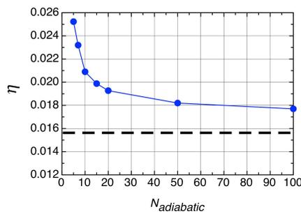
Figure 4: (blue) optimal starting values of parameter  $\eta$ , Eq. (4), versus number of FODO periods for adiabatic decline of duodecapole component, (dotted) the value of  $\eta$  for the channel with constant duodecapole component.
