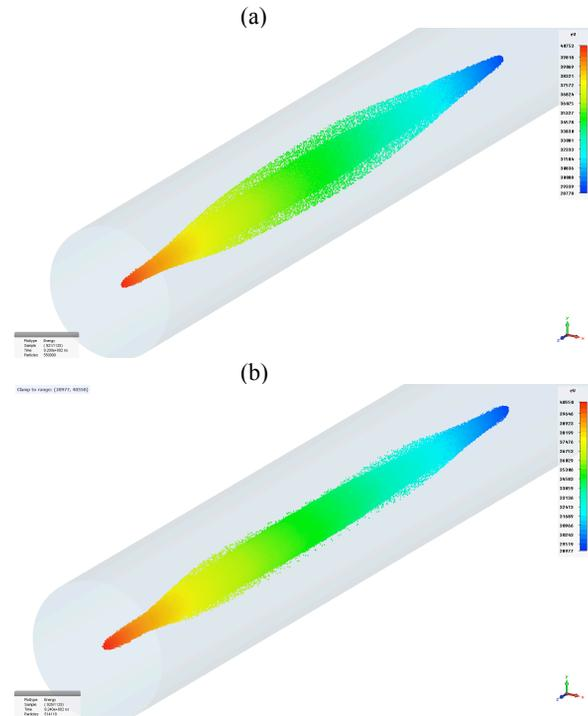
Figure 3: Final 3D distributions of the beam in 30 periods of (a) quadrupole channel, (b) quadrupole-duodecapole channel.
