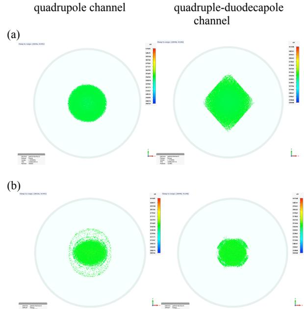
Figure 2: (a) initial and (b) final x-y particle distributions in a focusing channels containing 30 focusing FODO periods.
