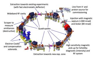
Figure 2: Sketch of the ELENA ring highlighting main features and particularities.
