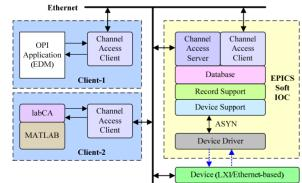
Figure 2: Software block diagram of building EPICS support for communicating with LXI/Ethernet-based devices.
