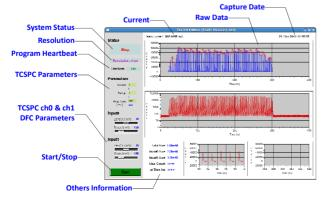
Figure 5: Layout of the TCSPC EDM page.
