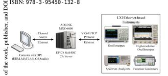
Figure 1: System architecture of building EPICS waveform support environment with LXI/Ethernet-based instruments.
