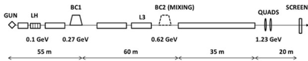
Figure 1. Sketch of the FERMI linac (not to scale) for the phase mixing experiment [10].
