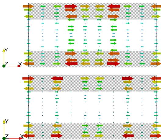
Figure 4: Electric field of a dielectrically lined rectangular waveguide with a point charge passing centrally through it. In the upper panel, the charge is located at  $z = L/2$ , in the lower at  $z = 3L/4$ .
