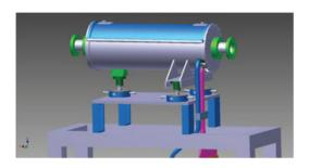
Figure 3: Quadrupole lens with ceramic tub and supply conductors mounted on the frame.(Picture: GSI).
