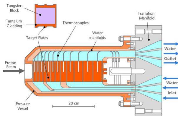
Figure 1: Layout of the ISIS-TS1 spallation target.
