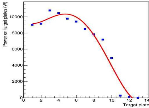
Figure 3: Total heat rate deposition onto the tungsten plates.
