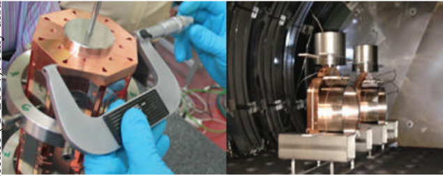
Figure 3: Dimensional checking during bars assembly (left) and compact couplers vacuum brazing (right).
