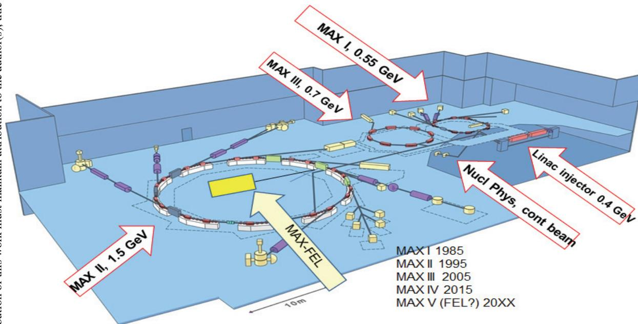
Figure 1: The MAX-lab facility.
