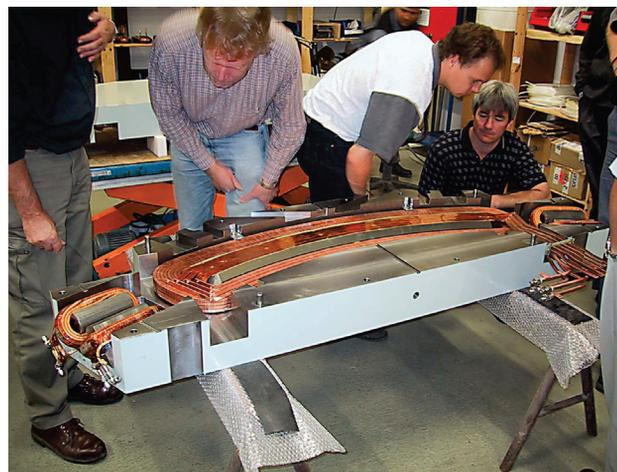
Figure 5: Half of a MAX III magnet block.
