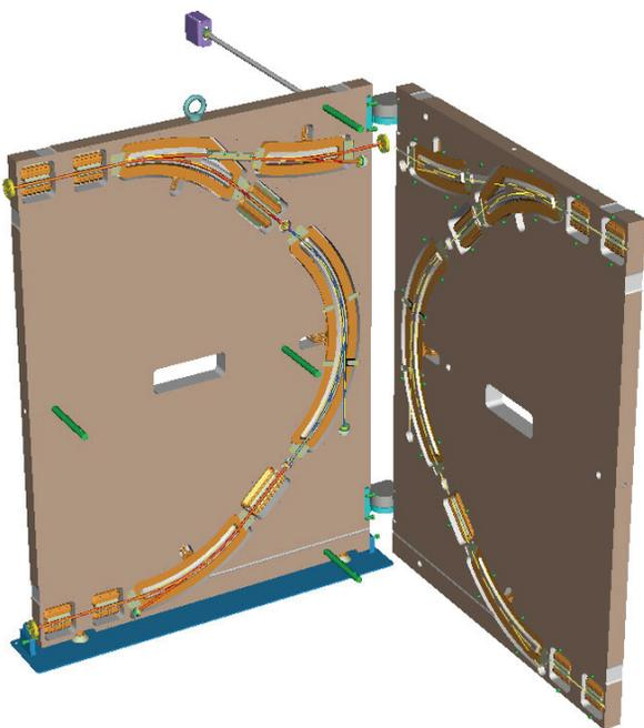
Figure 4: A MAX-injector isochronous achromat.
