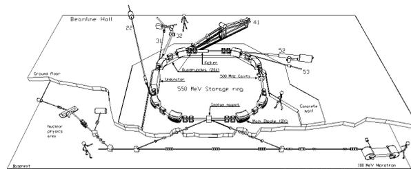
Figure 2: The MAX I accelerator. (Graphics from 1985).
