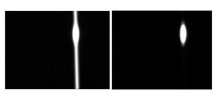
Figure 6: Enhanced frame before and after vertical smear removal.
