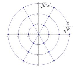
Figure 2: Example of the polar mesh.
