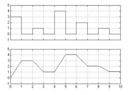
Figure 4: The integrator model in Simulink. Input signal (the 1st diagram) and output signal (the 2nd diagram). T11 0 D
