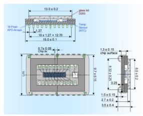
Figure 2: Package of AA16-0.13-9 APD linear array.
