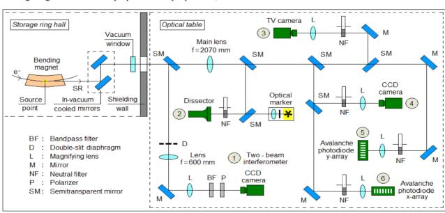
Figure 1: Layout of the optical observation station measurement part at SIBERIA-2 storage ring.
