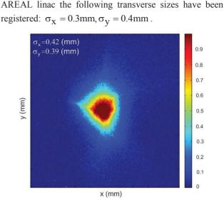
Figure 5: Electron beam transverse profile.
