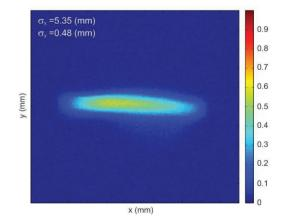
Figure 6: Electron beam transverse profile at the spectrometer YAG screens.
