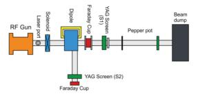
Figure 1: Layout of AREAL gun section with diagnostics.
