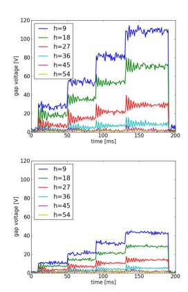
terms of the CC BY 3.0 licence (© 2014). Any distribution of this work must maintain attribution to the author(s), title of the work, publisher, and DOI Figure 4: Harmonic components of the gap voltage, (top) without fast rf feedback and (bottom) with feedback.
