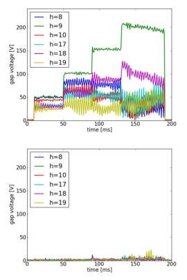
Figure 5: Harmonic components of the gap voltage, (top) without feedforward and (bottom) with feedforward.
