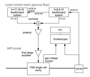
Figure 2: Schematic diagram of the beam test setup.
