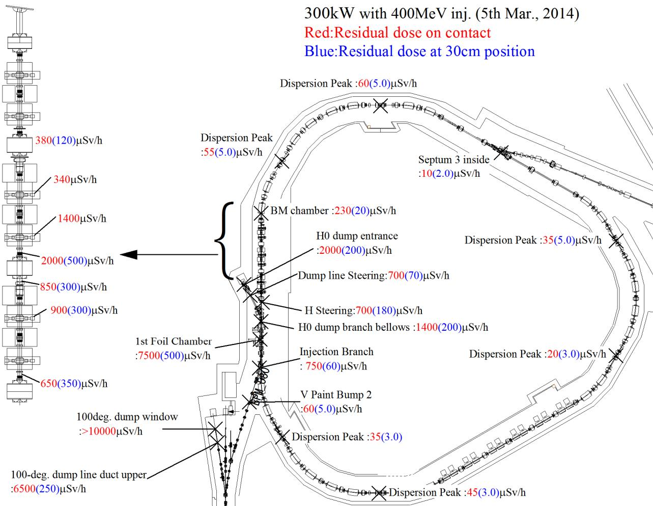
Figure 1: Residual dose distribution at 300kW operation with injection energy of 400 MeV. A left(red) value means a contact dose rate and a right(blue) value in bracket means a dose at “one-foot”(30cm from a vacuum chamber surface) position.
