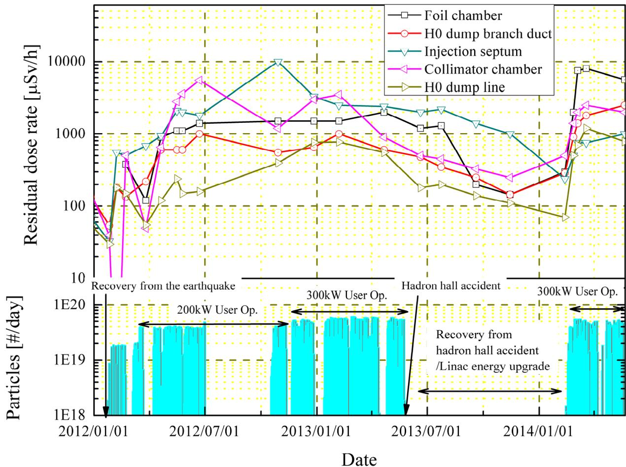
Figure 2: The history of the residual dose of typical loss point and output power of RCS.
