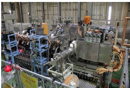
Figure 2: Test stand of the 50-mA ion source and RFQ.
