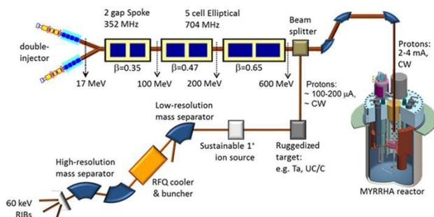
Figure 1: Layout of the MYRRHA proton driver.
