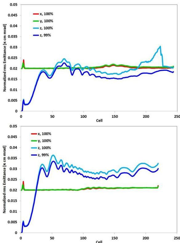
Figure 3: Emittance evolution along the RFQ (top: CZ2013; bottom: CZ2011).
