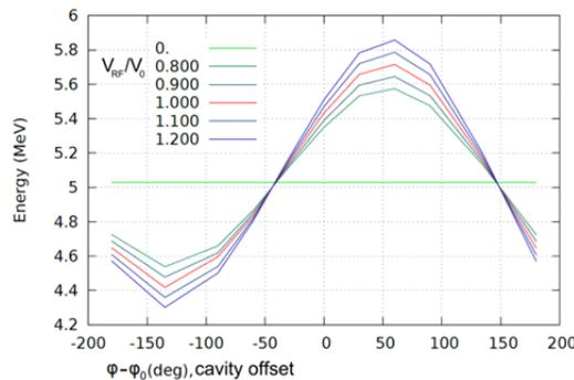
Figure 4: Energy signature for the first cavity.
