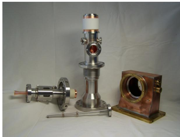
Figure 3: ILC coaxial input coupler.
