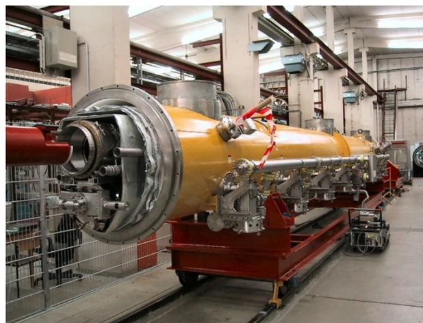
Figure 1: 1.3 GHz cavity cryomodule at DESY.
