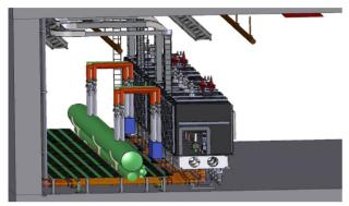
Figure 4: FRIB cryomodule with U-tube connections.
