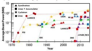
Figure 2: Achieved beam power at some major hadron facilities. Upgrade plans exist for most facilities.
