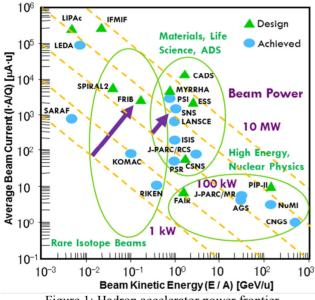
Figure 1: Hadron accelerator power frontier.
