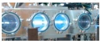
Figure 5: Test of He gas charge stripper using Uranium beams at RIKEN [39].
