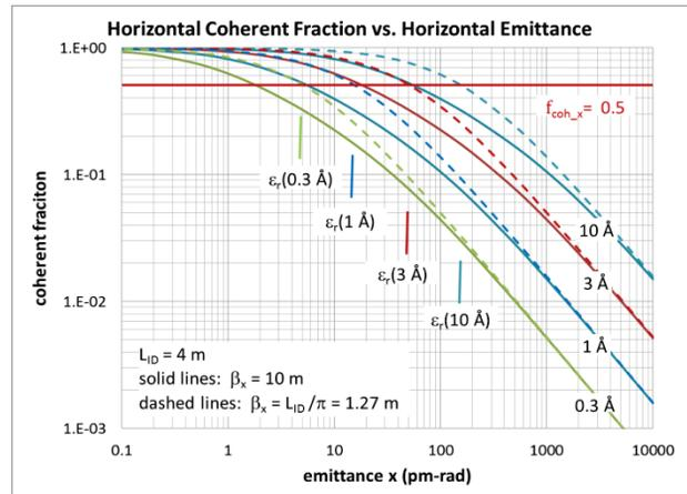
Figure 1: Horizontal coherent fraction vs. emittance (from Eqs. 5 and 8) for various X-ray wavelengths, with enhancement when  $\beta = L/\pi$ .
