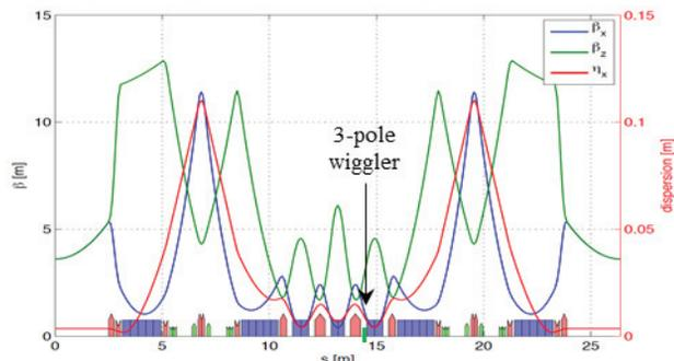
Figure 2: A 2013 version of a 7BA lattice for the ESRF with dispersion bumps and gradient dipoles (1,2,4,7).
