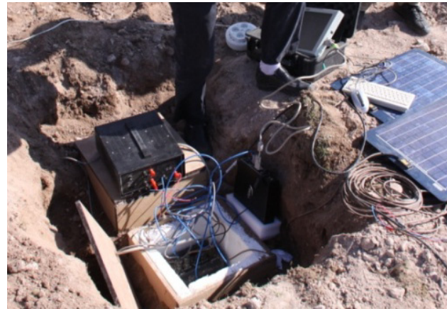
Figure 4: Installation of seismometer.
