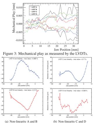
Figure 4: Non-linearities in the LVDT measurements.
