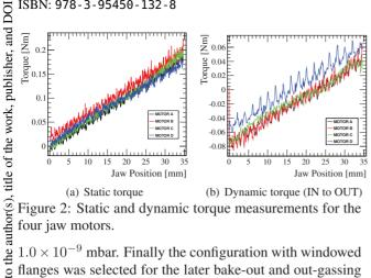
Figure 2: Static and dynamic torque measurements for the four jaw motors.
