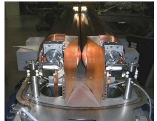
Figure 1: Photo of the upbeam, rotation drive, end of the RC before the vacuum tank cover is installed and welded.
